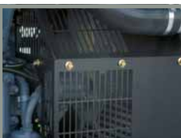
Moving and rotating parts protection
